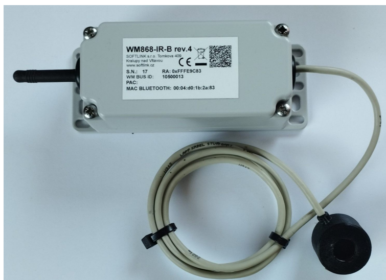
Figure 13: View of the WM868-IR-B module with connected antenna and optical head
