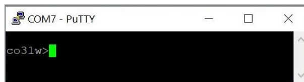
Figure 6: Open terminal window for module configuration via serial line
