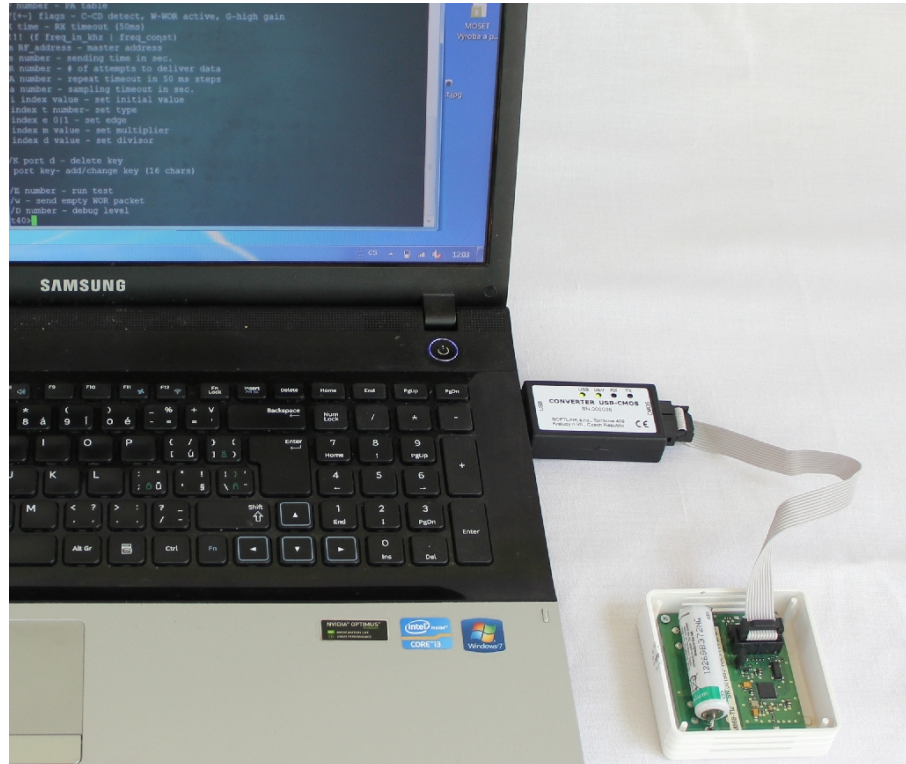
Figure 4: Configuration via USB port of computer
