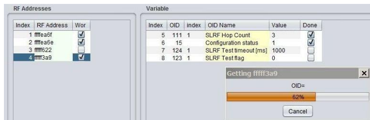
Figure 16: Progress of getting values of preselected variables of the module by using of „GET“ command
