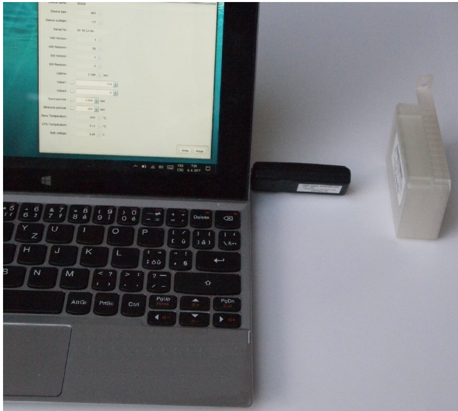
Figure 7: Configuration of the module with using of optical converter
