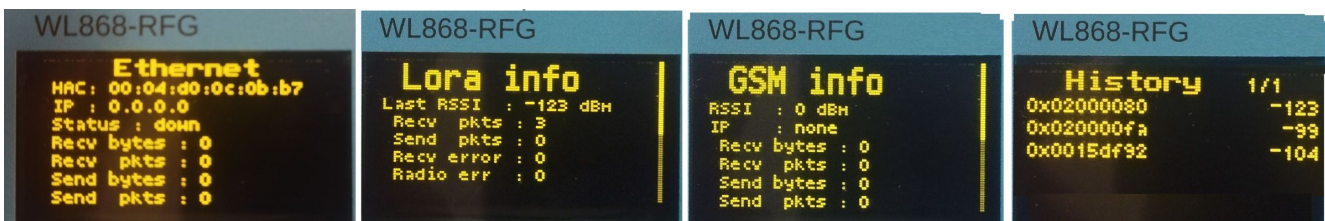
Figure 6: Preview of Ethernet, LoRa, GSM and History menu item displays
