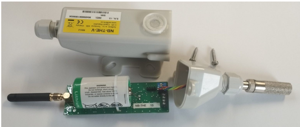
Figure 7: Assembly of NB-THE-V module with rod antenna
