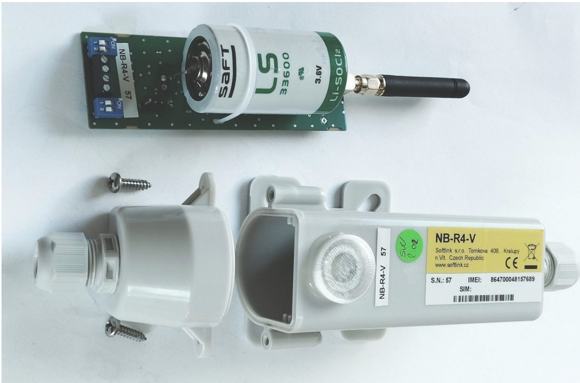
Figure 6: Assembly of the NB-R4-V module with a rod antenna
