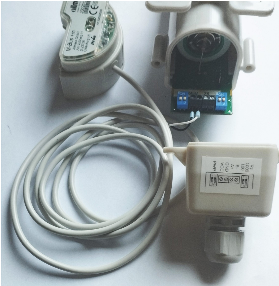
Figure 8: Connection of a meter with RS-485 output to the NB-R4-V module terminal block
