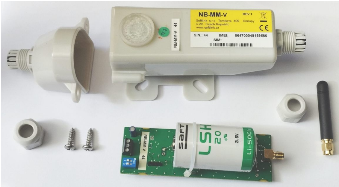
Figure 6: NB-MM-V module assembly with stick antenna
