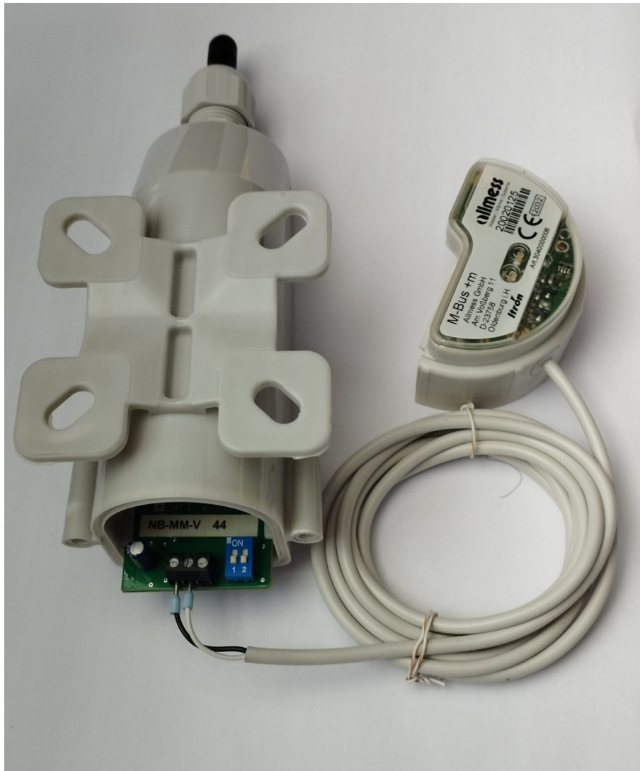
Figure 8: Connection of a meter with M-Bus output to the NB-MM-V module terminal block
