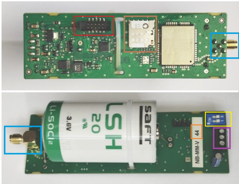
Figure 7: Detail of NB-MM-V module printed circuit board
