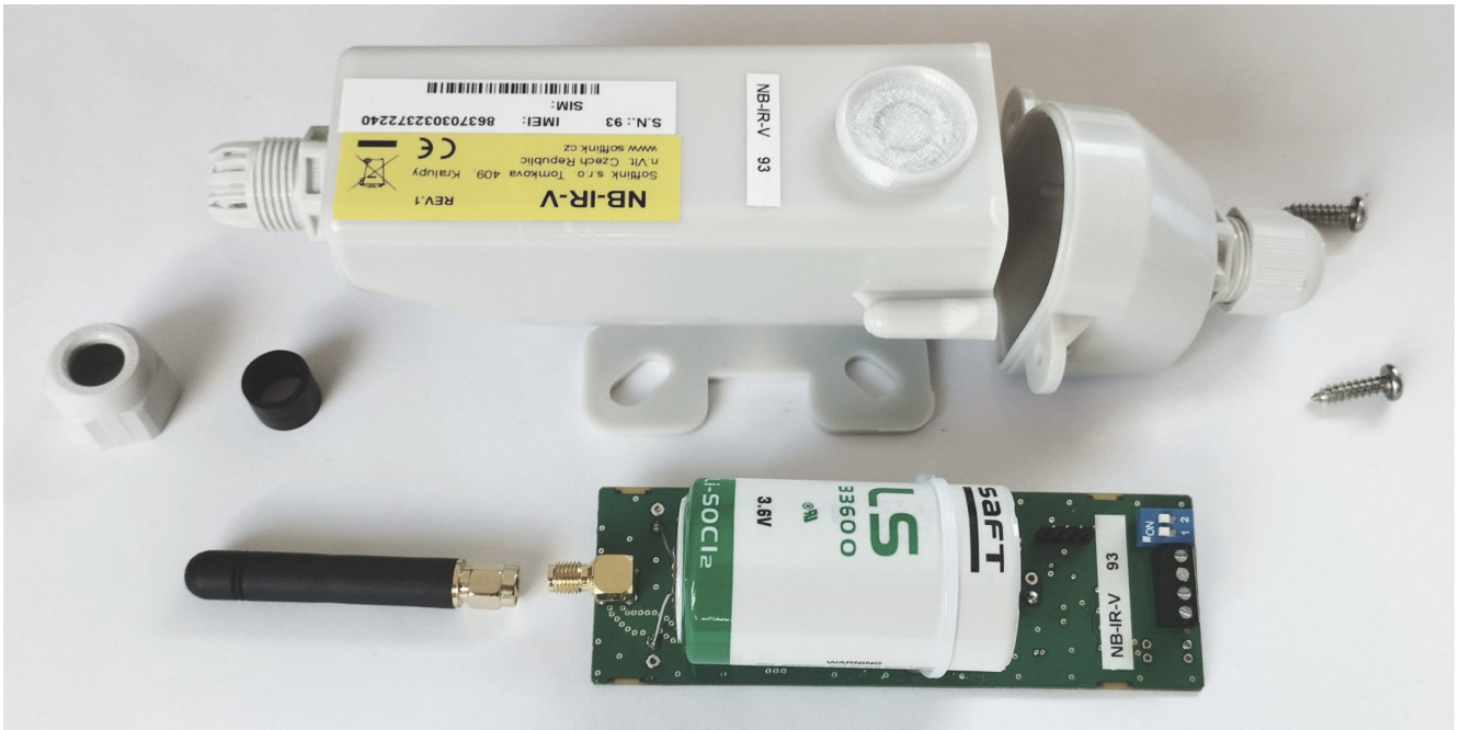
Figure 6: Assembly of the NB-IR-V module with a rod antenna
