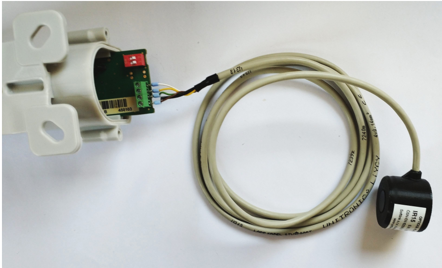
Figure 8: Connecting the optical head to the NB-IR-V module terminal block
