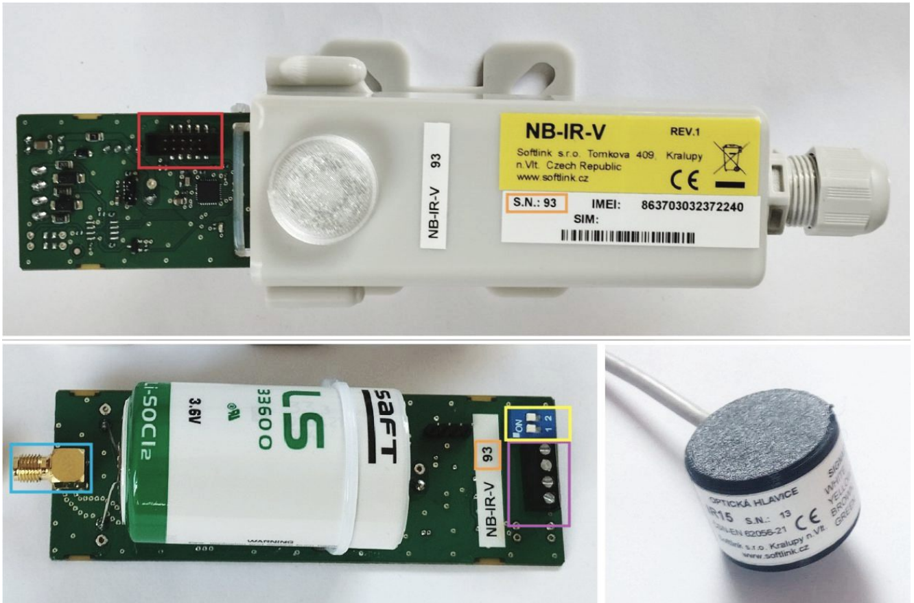
Figure 7: Detail of the NB-IR-V module printed circuit board
