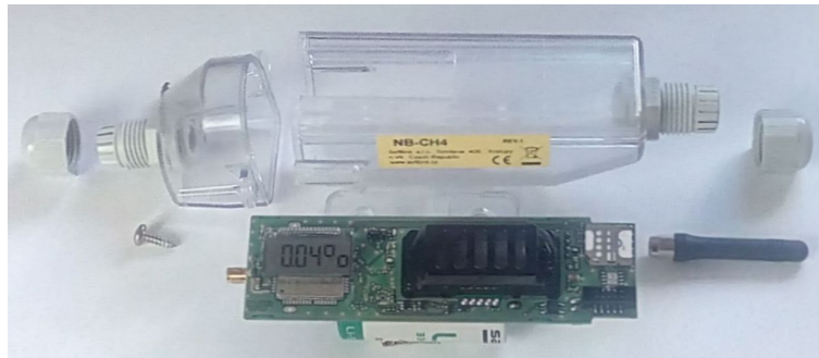
Figure 6: Assembly of NB-CH4 module with stick antenna
