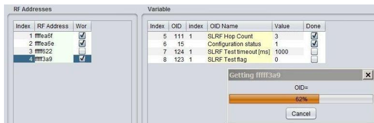
Figure 11: Progress of getting values of preselected variables of the module by using of „GET“ command
