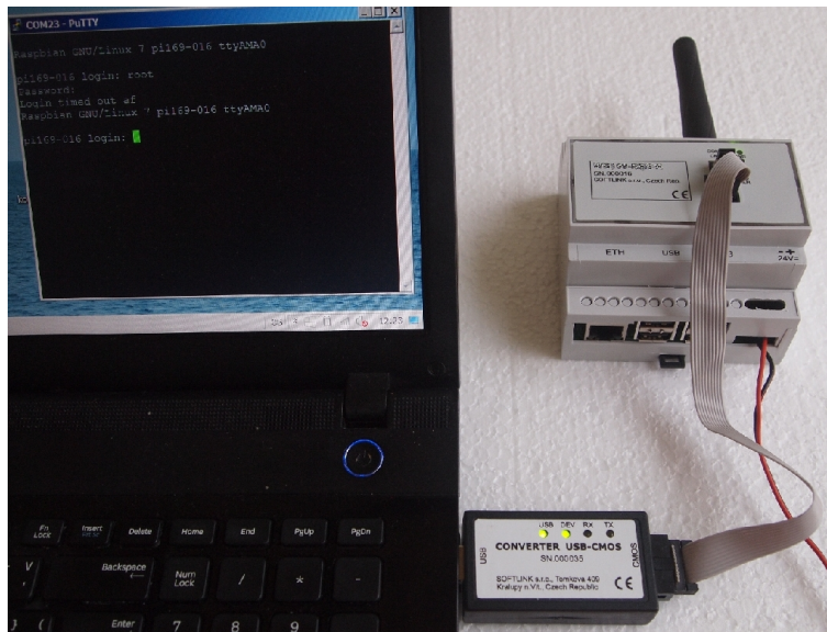
Figure 4: Configuration via USB port of computer
