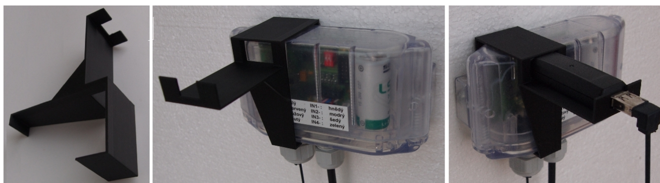
Figure 12: Attaching of optical converter to the holder
