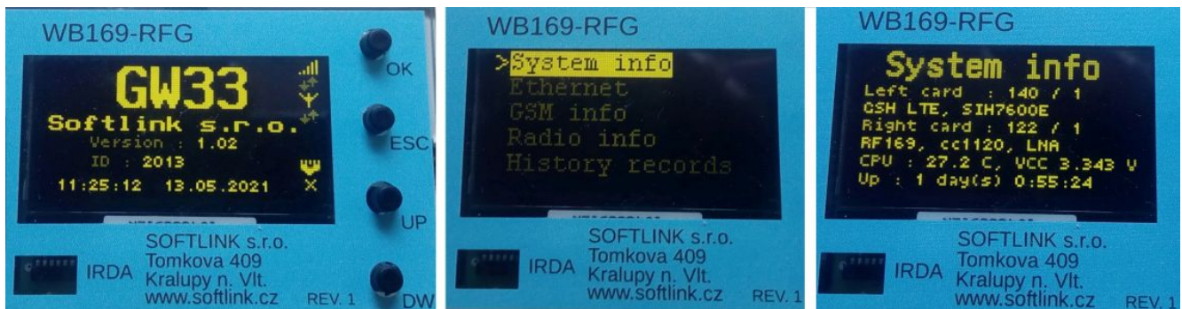
Figure 5: Display the main screen, main menu and system information
