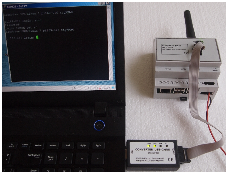
Figure 3: Configuration via USB port of computer
