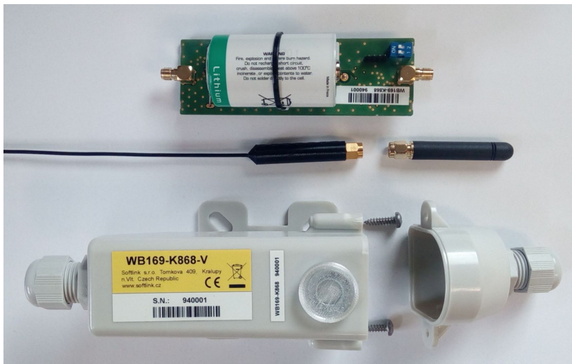
Figure 10: Set of WB169-K868 module components with rod antenna
