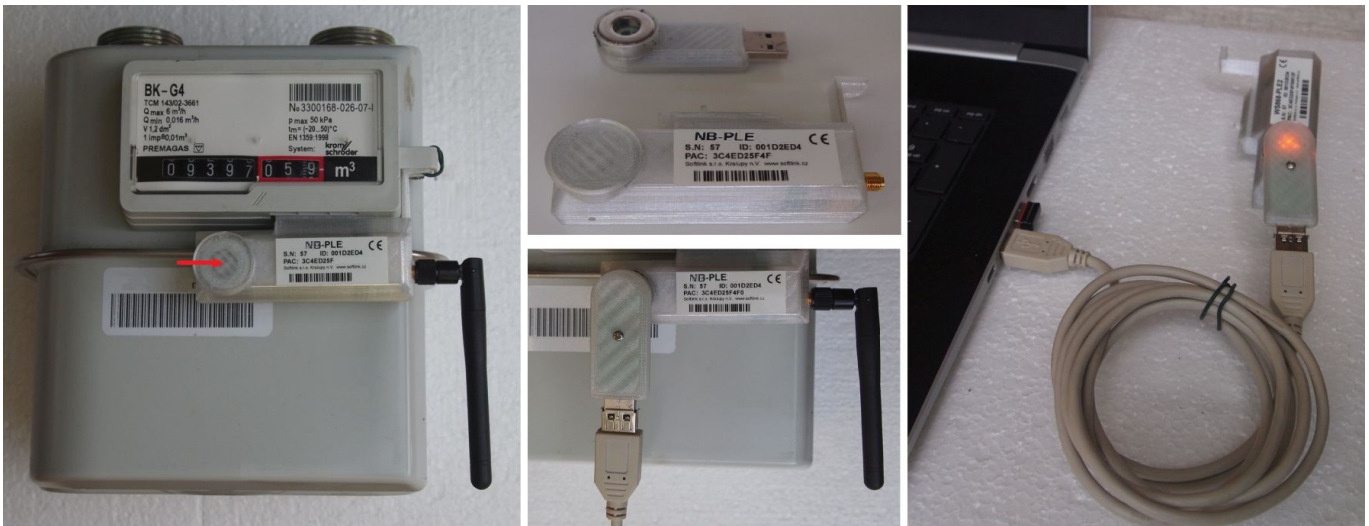
Figure 11: Installation and setting of NB-PLE module
