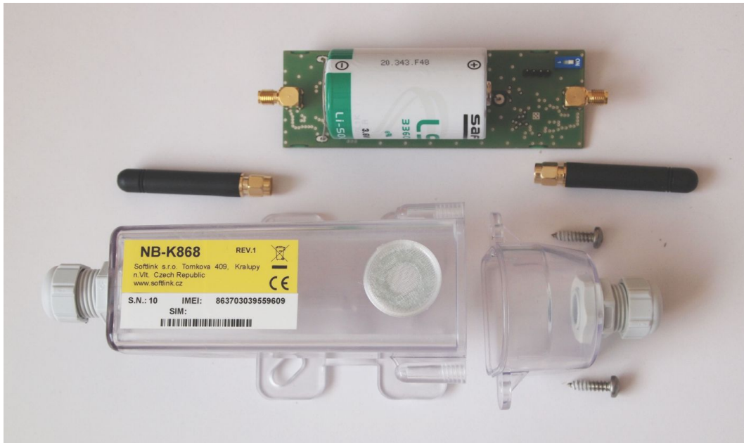
Figure 7: Set of NB-K868 module components with stick antenna
