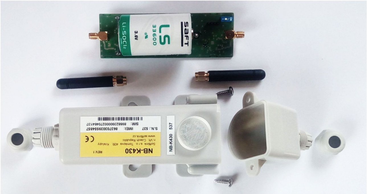
Figure 7: Set of NB-K430 module components with stick antenna
